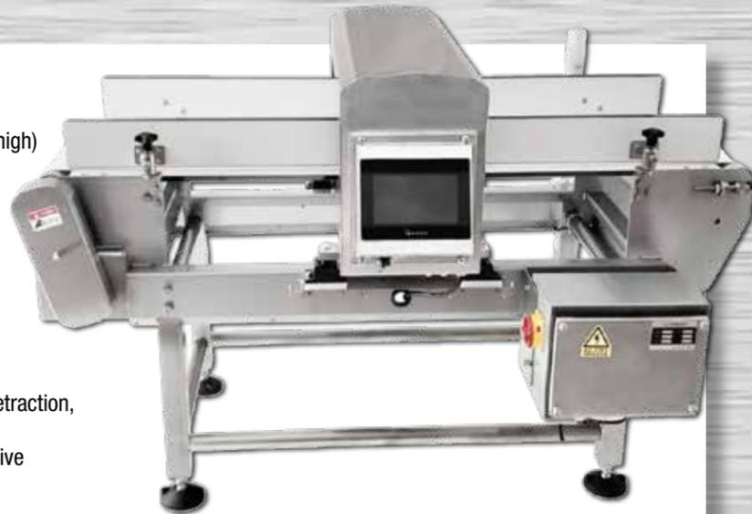
The **MD-SR Series** of IP65 metal detectors are specifically designed for high demand of sensitivity, stability and intelligent detection. Utilizing a patented self-adaptable algorithm plus the combination of the well-known industrial components, integrated circuits and ARM processor+FPGA motion control computations, the **MD-SR Series** metal detectors lead detecting performance in the industry.
